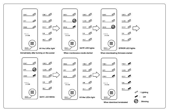
Figure 4.2 Downloading firmware in the maintenance mode
